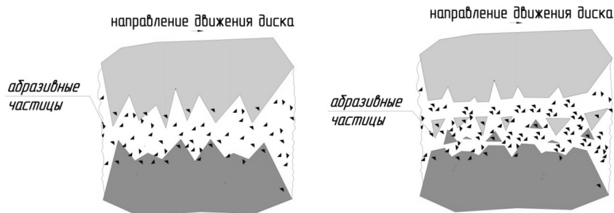
Figure 6 – The scheme of operation without lubrication
