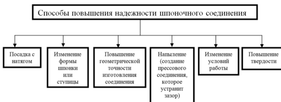
Figure 2 – Methods of improving the reliability of the keyway
