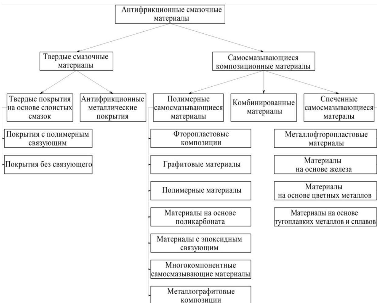
Figure 5 – Antifriction lubricants and coating for units of dry friction
